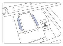
There is a wireless cellular phone charging system in front of the cup holders. The system operates with all doors closed, and the Engine Start/Stop button in the ACC/ON/START position.
